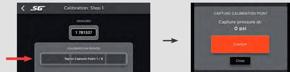
2. Tap on the next grey icon. Generate the exact specified pressure, ensuring it settles for at least 1-2 seconds and tap 'Capture'.
