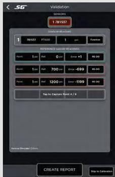
Alternatively, if you have a mix of PASS and FAIL sensors in one verification, you can finish the verification process. On the report page, enter comments for the PASS sensors and tap 'CALIBRATE FAILED SENSORS'. This will finalise the PASS reports, and start a calibration with only the FAIL sensors. POWER OFF the PASS sensors before starting calibration.
