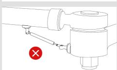
The sensor should be in the centre of its movement. (Showing close to 25mm on the MultiTool Pro).
