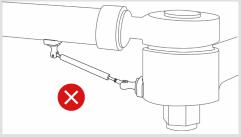
The sensor should be in the centre of its movement. (Showing close to 25mm on the MultiTool Pro).
